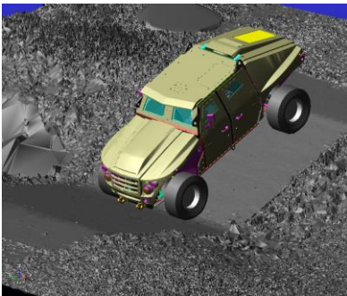
Figure 4-21: Ditch Crossing, 3D discretized road approach
