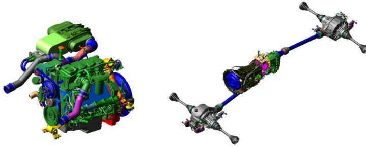
Figure 2-10: Powertrain and Driveline system
