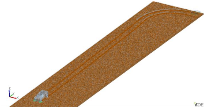
Figure 6-10: EDEM Fine Grain Wet sand Simulation
